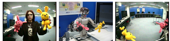
Figure 1: Setup for the imitation experiments between Infanoid and a human experimenter. In the left image, the human subject holds the two coloured object in each hand, trying to imitate the robot that is performing random arm movements. In the center image, the robot is displayed holding the two coloured objects by itself, also performing random arm movements. The right image shows the objects as seen by the robot.
